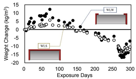
Fig. 6: Comparison of weight change measured of series WLW and WLS.
