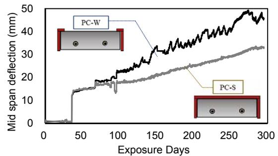
Fig. 8: Comparison PC slabs deflections measured.
