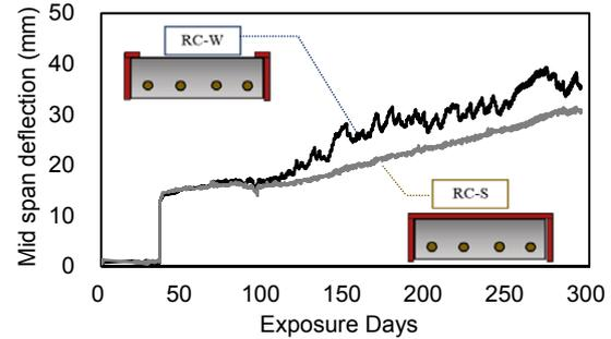
Fig. 7: Comparison of RC slabs deflections measured.
