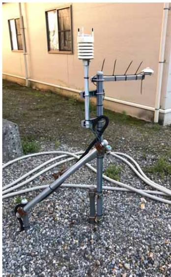
**Fig. 4:** Weather station located at exposure test site.
