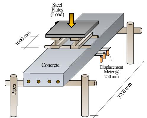
**Fig. 3:** Exposure-load test layout.
