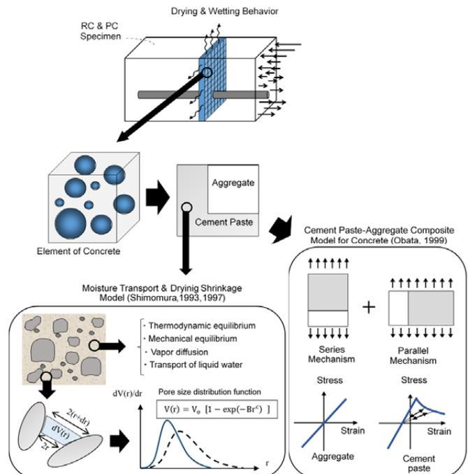
Fig. 9: Outline of computational model employed for hygrothermal and stress analysis.
