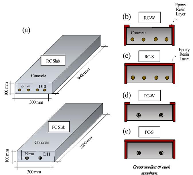
**Fig. 1:** Specimen dimensions and seal conditions details.
