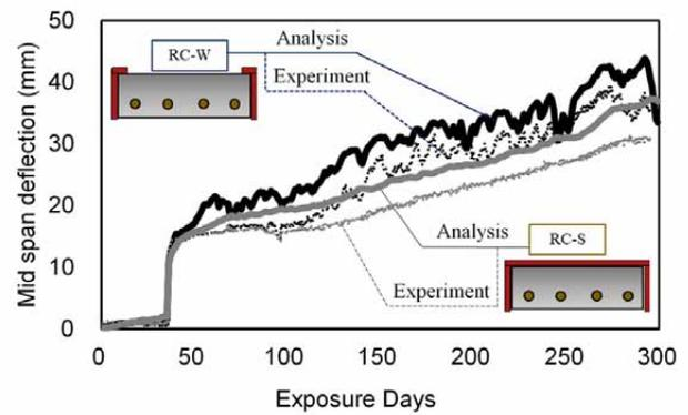
Fig. 10: Comparison of analytical results and experimental data of RC slabs deflections.
