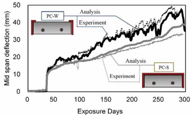
Fig. 11: Comparison of analytical result and experimental data of PC slabs deflections.
